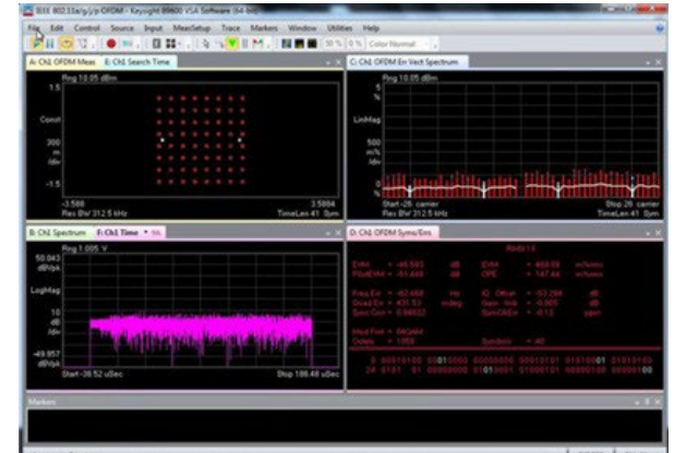
Using data acquired from S-Series, VSA shows an EVM for IEEE 802.11 QAM 64 of 0.47%.
